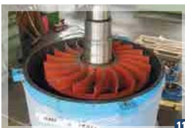
11 Rimontaggio pompa. Vacuum pump assembly.
