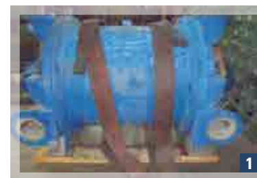
1 Pompa da revisionare tipo Nash 904. Vacuum pump to repair type Nash 904.
