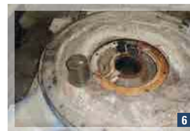
6 Testata intasata. Clogged end shield.
