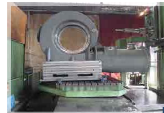
7 Parte stampo cerchio in lega auto. Mechanical machining - alloy wheels for car(part of mold).
